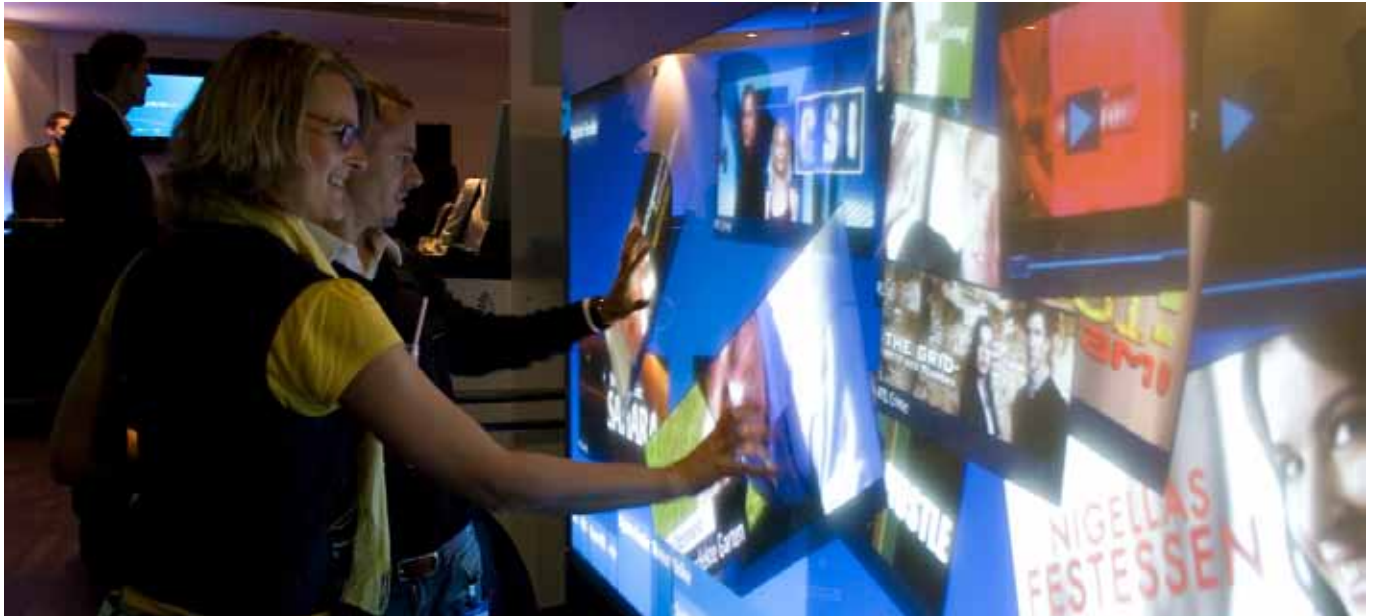
A multiuser multitouch back-projection box (3 meters long, 2 meters high) and the application developed for IP Deutschland.
